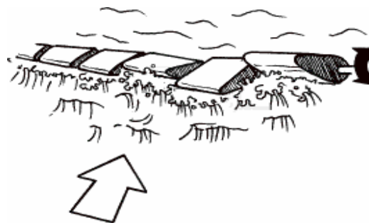
Fig. 5 Concept of Salter Duck WEC [8]
