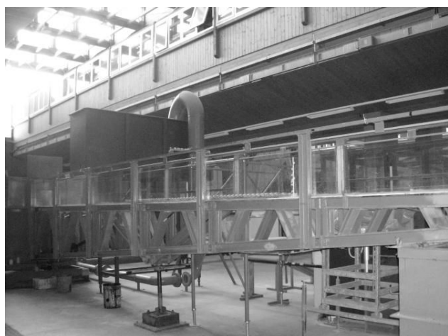
Fig. 1 View of the free surface open channel
