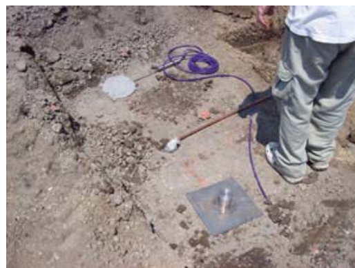
Fig. 7 OSU pavement instrumentation installed at bottom of FDR layer (left to right) — pressure cell, pore pressure device and LVDT base
