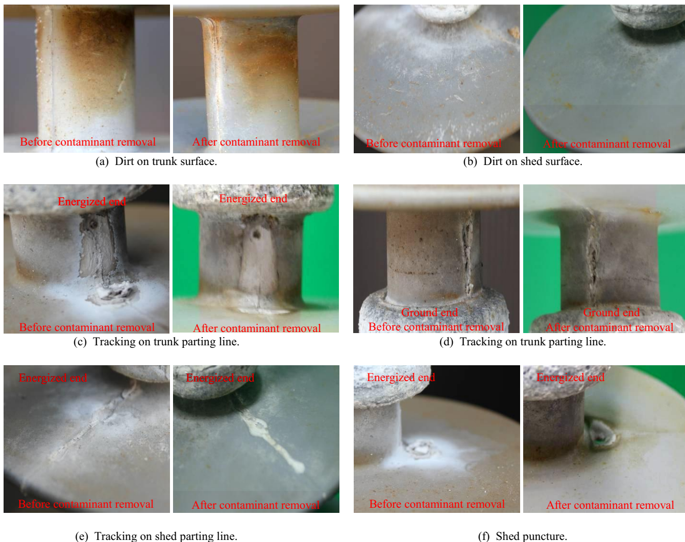
Fig. 5 Surface damage of tested specimens.
