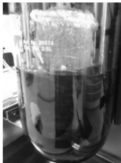
Fig. 4 Attachment of P. simplicissimum mycelium seen in the RFBB at the end of the fermentation process
