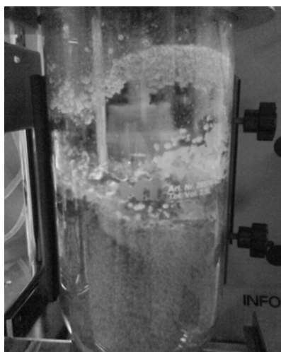
Fig. 3 Medium was filled with pellets and the filamentous fungus of freely suspended cells attached everywhere
