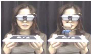
Fig. 1 augmentation based marker (left figure contains a marker, and the right shows the same scene after augmentation) [2]
