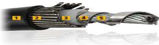
Fig. 4 Construction of Bowden cable 1) plastic sheathing 2) outer sheathing made of spring steel wire 3) Teflon guide sleeve 4) spiral wire 5) inner core made of spring steel wire [14]
