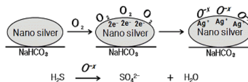
Fig. 1 Mechanism of inorganic compounds oxidation on silver nano-surface
