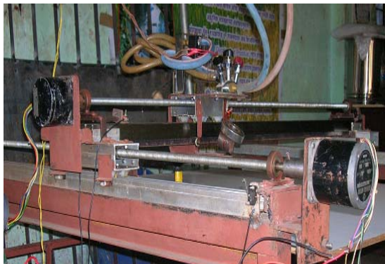
Fig. 5 Stepper motor mounted on the setup
