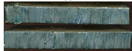
Fig. 10(a) 100 x 65 rectangular hole (b) Rectangular hole cutting (Manual) (c) Cutting edge obtain in manual cutting
