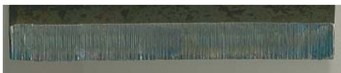
Fig. 9 (a) 100 x 65 rectangular hole (b) Rectangular hole cutting (Automatic) (c) Cutting edge obtain in automatic
