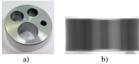
Fig. 1 The specimen (a) and X-ray projection (b)
