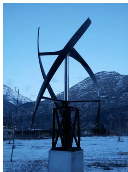
Fig. 1: VAWT tested in Longarone open wind facility, BL (Italy)
