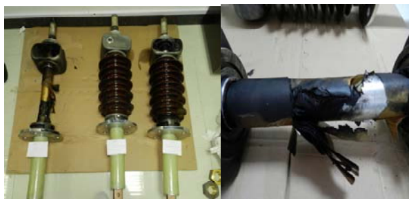
Fig. 1 Photo of three failed transformer bushings
