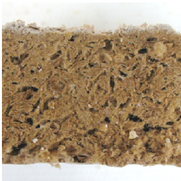
Fig. 3 Porous matrix obtained with 30% of \text{NaHCO}_3
