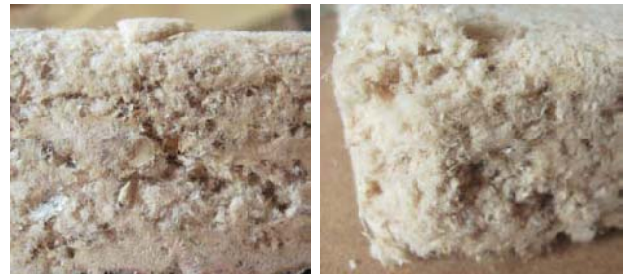
Fig. 4 Soft fibrous panel made with cellulose flakes and PCMs
