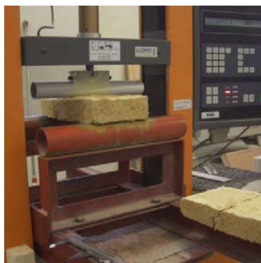
Fig. 9 Three points bending device used for mechanical Tests
