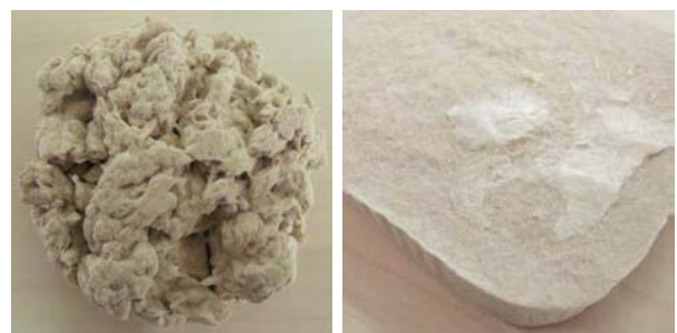
Fig. 6 Sample obtained with freeze-dry process
