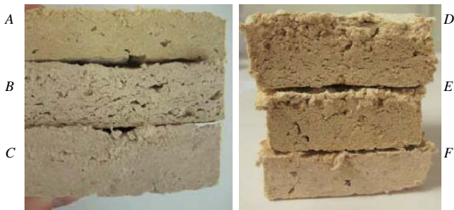
Fig. 2 Samples of panels obtained with rising agents. A and F without additives, B with brewer's yeast, C with baking powder, D with 30% of \text{NaHCO}_3 , E with 50% of \text{NaHCO}_3
