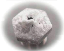
Fig. 3 Fouling of the nozzle injecting the binding solution
