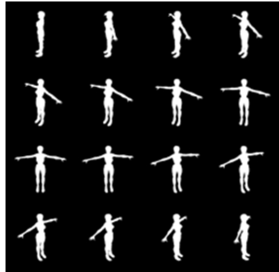
Fig. 2 Silhouette Images Captured by Pose Capture Module
