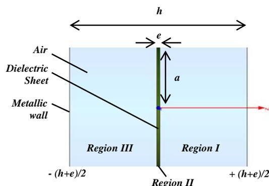
Fig. 2 Loaded cavity divided into three regions
