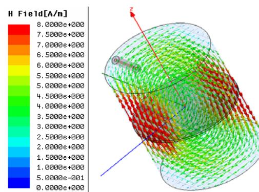
Fig. 9 H-field of TE<sub>111</sub> of unloaded cavity
