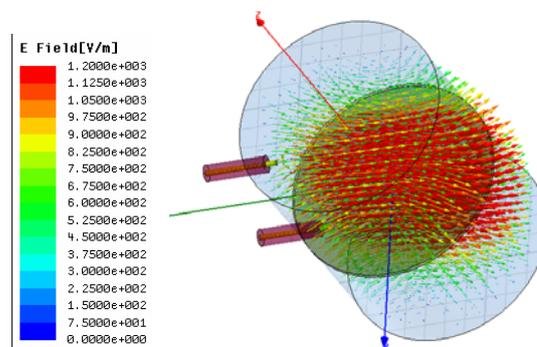
Fig. 8 E-field of TE<sub>111</sub> of unloaded cavity
