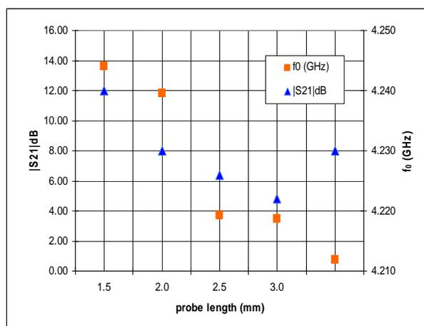
Fig. 6 Plot of |S21|dB and f<sub>0</sub> versus probe lengths
