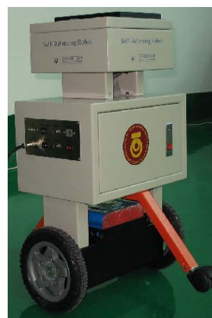
Fig. 1 The prototype T-WIP mobile robot
