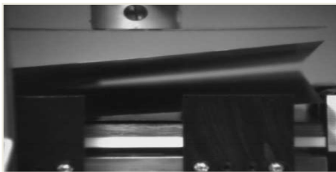
Fig. 7 Wafer lifting during picking process
