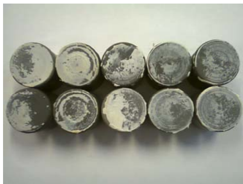
Fig. 6 bonding strength test sample after bond test
