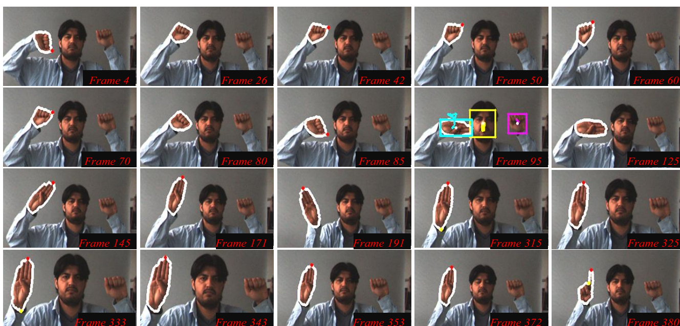
Fig. 6 Test Sequence "ABD-Sequence" for the postures signs 'A', 'B' and 'D' with different rotations, scaling and partial occlusion is presented.
