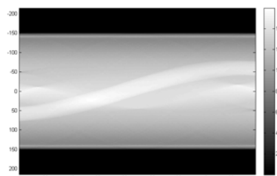
Fig. 6 Sinogram of the specimen with defects
