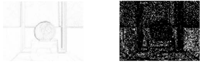
Fig. 2. The left-hand image is an EPP (Error Per Pixel) image: This image can be used to indicate to a user the locations within the scene which contain more errors. The right-hand image is an NPP Image: This image can be used to indicate which locations can be reconstructed exactly
