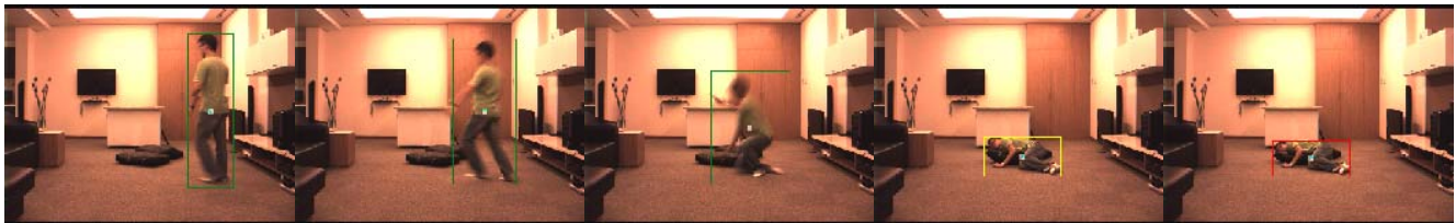
(a) Object standing, aspect ratio > 1 (b) Object starts falling, aspect ratio > 1 (c) Object falling, aspect ratio > 1 (d) Object lie on the floor, aspect ratio < 1 (e) Inactivity period over, fall confirmed
