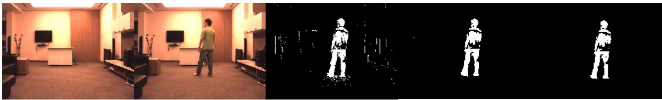
(a) Background frame (b) Incoming frame (c) Background subtraction (d) Median Filtering (e) Morphological process
