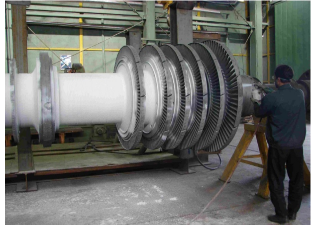
Fig. 3 Spraying calcium carbonate solution over the rotor surface
