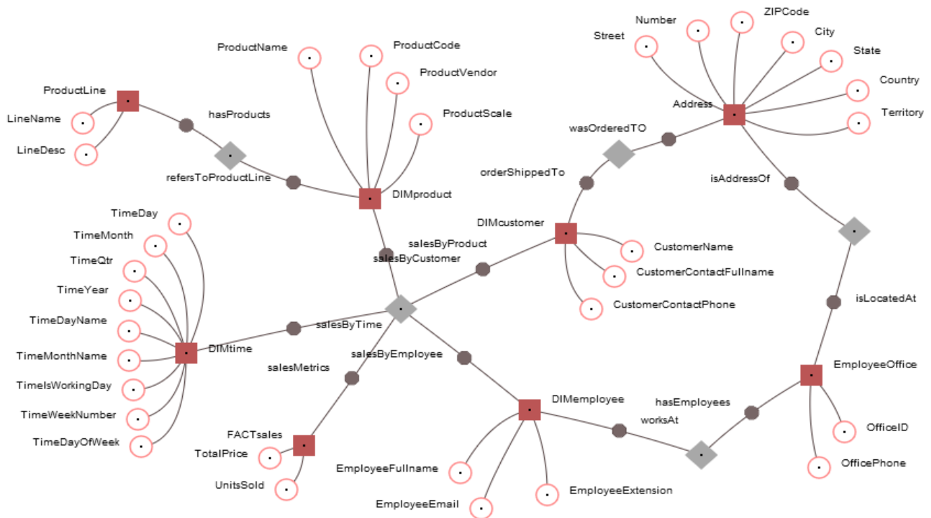
Fig. 4 Initial STAR schema converted into a more decomposed anchor model
