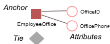
Fig. 1 Visual representation of anchor model's components
