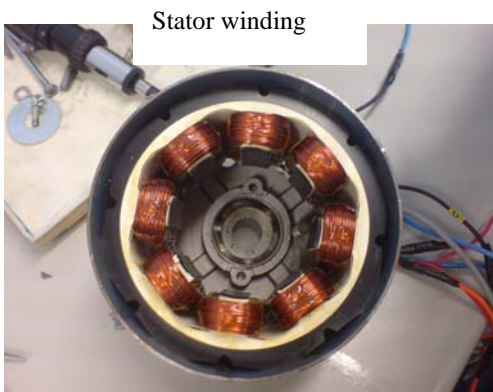
Fig. 1 4 phases SRG stator poles and winding
