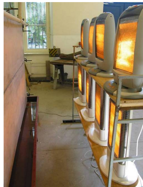
Fig. 3 Warming glass-fiber-concrete façade panel: view to electric warm sources and water tub
