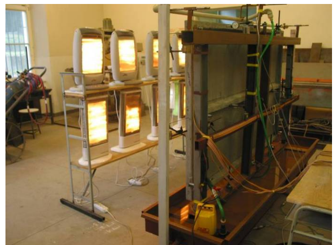
Fig. 4 Warming glass-fiber-concrete façade panel: view to panel backside with installed detectors
