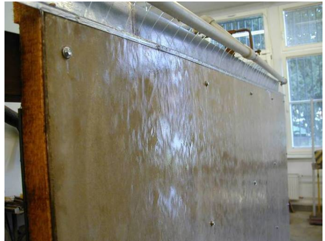
Fig. 18 Sprinkling fiber-cement slabs: view to water out flowing from sprinkling tube
