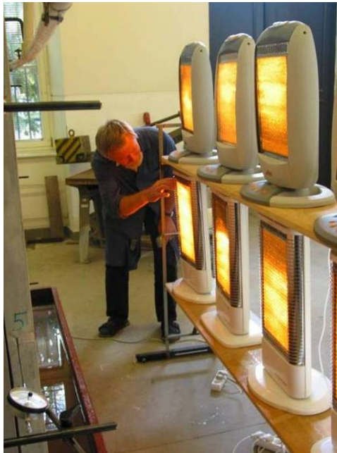
Fig. 15 Warming fiber-cement slab: preparation of equipment
