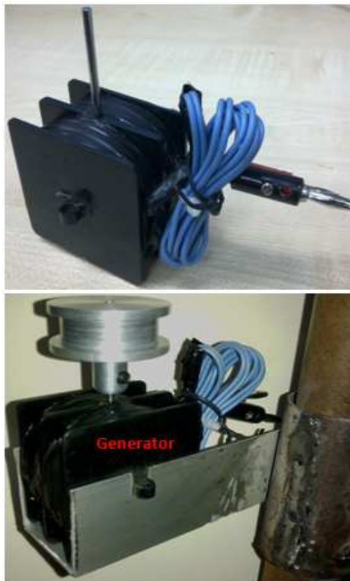
Fig. 3 In-house Production of AC Generator
