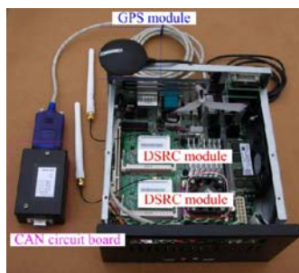
Fig. 13: Test platform, including DSRC, GPS and CAN board.
