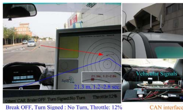
Fig. 16: Remote warning test in short range.
