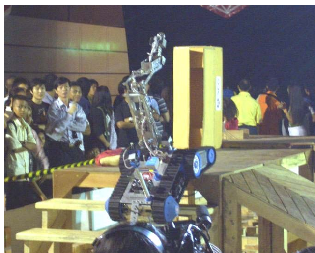
Fig. 1 The CEO Mission II, rescue robot with multi-joint mechanical arm in the Thailand Rescue Robot Championship 2006
