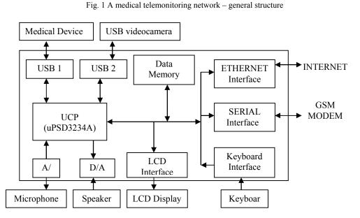
Fig. 2 The biosignal / ECG telemonitoring unit of our project
