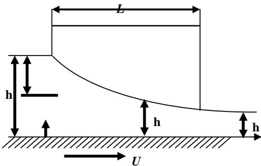
Fig. 1 Bearing geometry of a parabolic shaped slider
