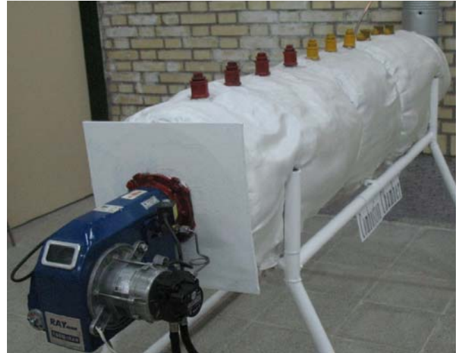
Fig. 2. Laboratory combustion chamber
