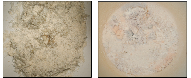
Fig. 8 Solidified glass melts with ash residuals from burning wheat and ray straw
