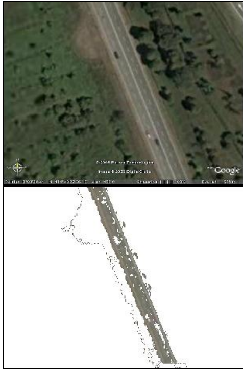
Fig. 4 Extraction on a straight road
