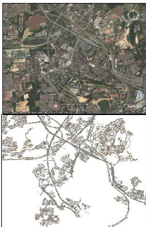
Fig. 8 Extraction on large scale complex road
