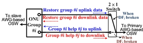
Fig.8. Four operation modes in 2 \times 1 optical switch
