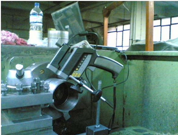
Fig. 8 Infrared camera installation on the lathe
