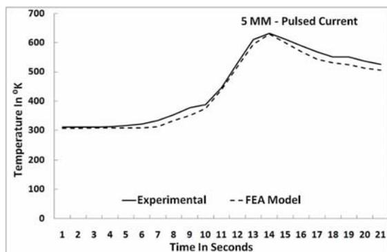
Fig. 7 (a) Experimental Vs FEA at 5 mm Pulsed Current
