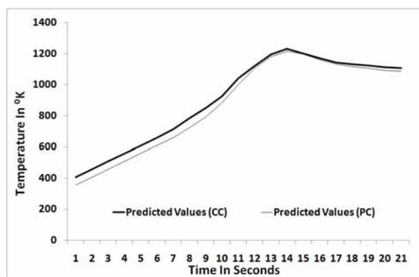
Fig. 9. Predicted values of temperature at weld centre
