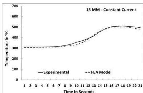
Fig. 8 (b) Experimental Vs FEA at 15 mm Constant Current
