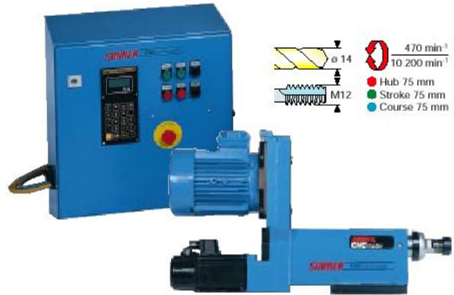
Fig. 3 A CNC machining unit with its controller [1].
