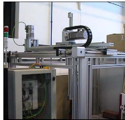
Fig. 3. Robot obtained. Photo 2. (Structure, SIEMENS AC induction machines and control SIEMENS-MASTERDRIVE drivers)
