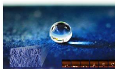
Fig. 4 Superhydrophobic surface fabricated by ZnO NWs with chemical modification [ref. 6]
