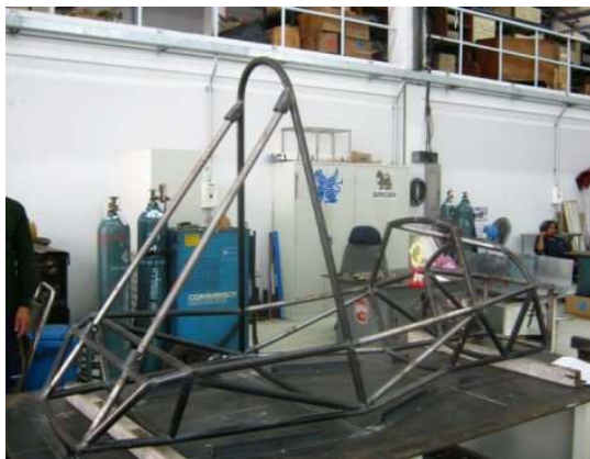
Fig. 3 The 2011 frame for 2011-2012 Auto Challenge student formula
