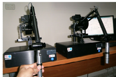
Fig. 7 bilateral teleoperation system using two Phantoms
