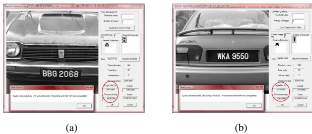
Fig. 9. Successful image results based on Heuristic Threshold, and MLP-BP classification techniques.
