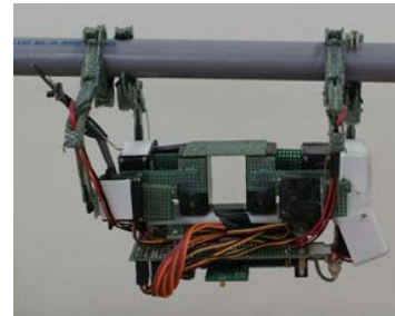
Fig. 10 Pipe crawling robot with a monitoring probe
