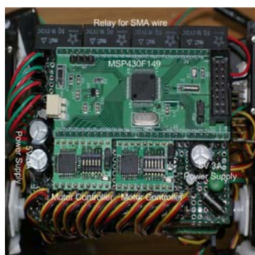
Fig. 6 A microcontroller unit for a pipe robot
