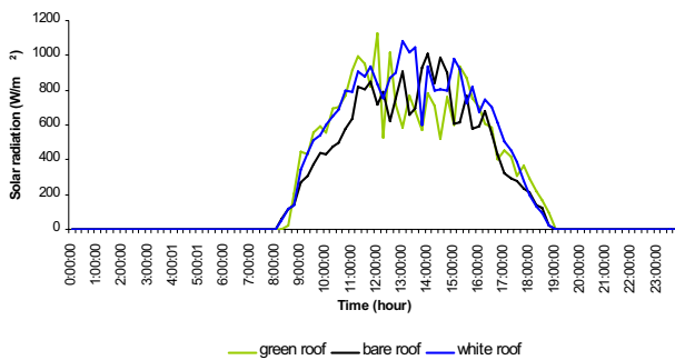
Fig. 5 Comparison of average solar radiation between black bare roof, green roof and white roof for six days' reading
