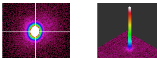
Fig. 13 profile of a TEM00 gaussian mode
