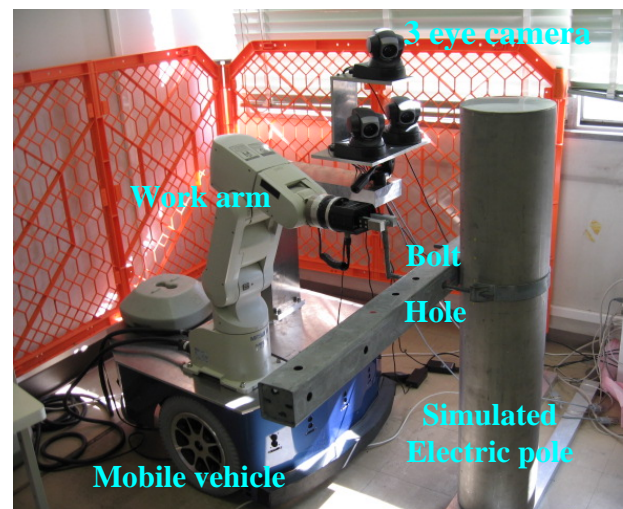
Fig. 1 Experimental power distribution line maintenance robot system
