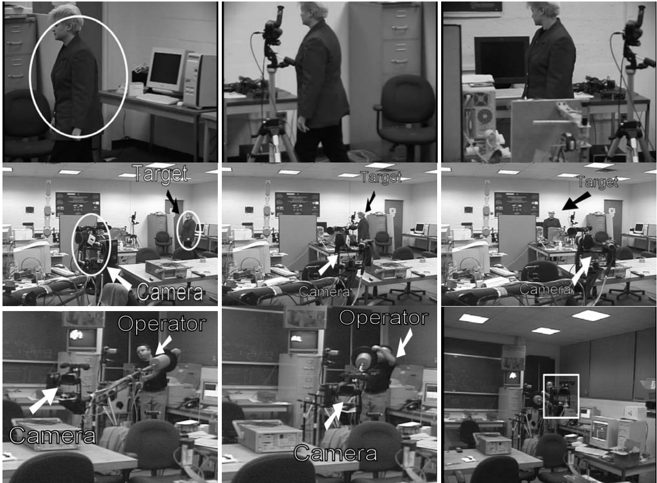
Fig. 3. Three sequential images from videotaping a tracking experiment. Camera field-of-view (top row) shows the target is kept centered in the image plane despite boom motions executed by the operator. Such motions are illustrated by the middle and bottom rows' images; two cameras placed in the room were used to record the experiment.
